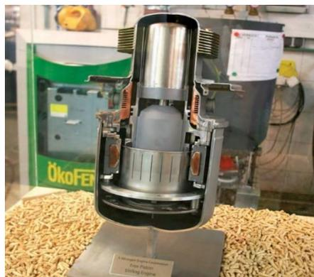
Figure 2.19 Stirling engine using biomass [10]
