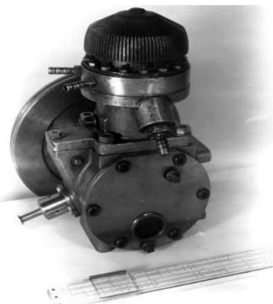
Figure 2.2 Single-cylinder Philips 2 h.p. Stirling engine
