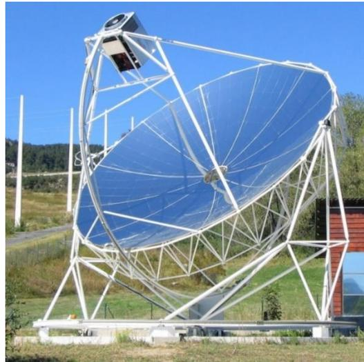
Figure 2.16 Solar powered dish Stirling engine
