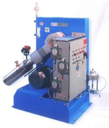
Figure 2.23 Cryocondensation pump
