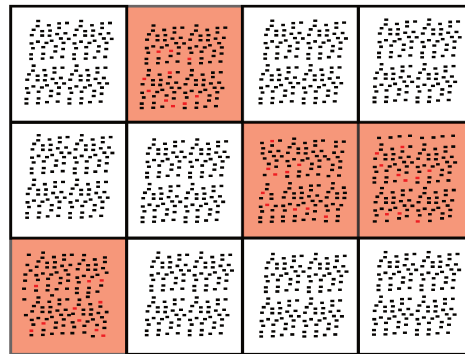
Fig. 5.1: Selection of a sample of size n = 40 in a population of units (black dots) divided in M = 12 primary units of equal size N_j = 64 , j = 1, \dots, M ( N = 768 ) with a two-stage design. First, a sample of m = 4 first-degree units are selected between the M = 12 with simple random sampling (in pink). Then in each of these 4 selected primary units, 10 units of the population are selected (red dots), again via simple random sampling.
