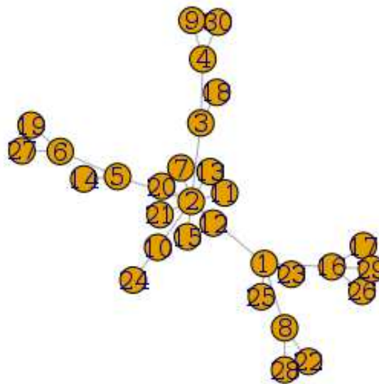
Fig. 6.15: Example of an undirected Barabási-Albert graph with 30 vertices. Vertices that appeared earlier (indicated by a low vertex index) have a higher attachment probability (and thus generally a higher degree). Mean degree for the graph is 1.93, kurtosis of the degree distribution is 10.4.
