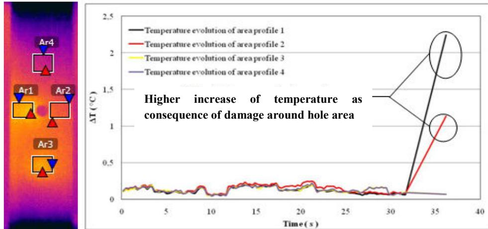
Figure 4.9 Temperature evolution of GFRP 90° with hole
