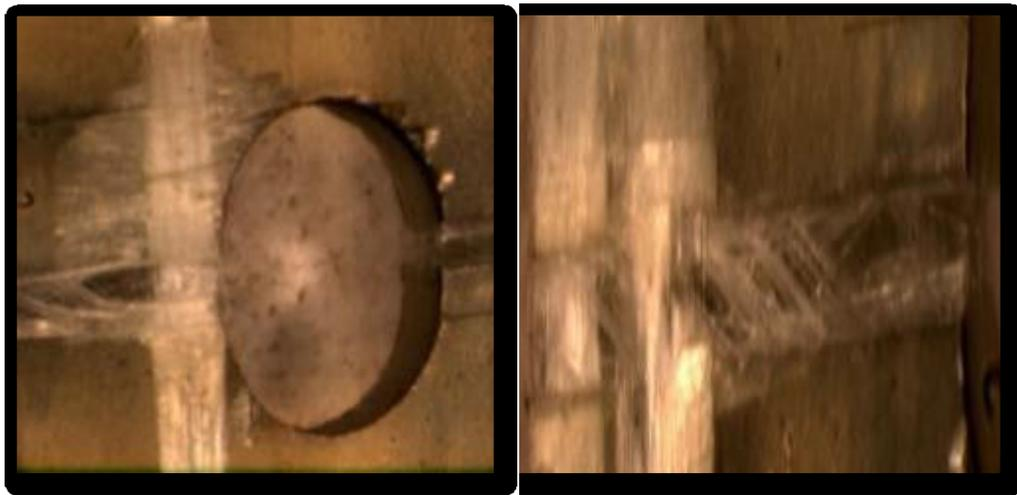
Figure 4.7 Microscopic observation on damage of GFRP 90° with hole
