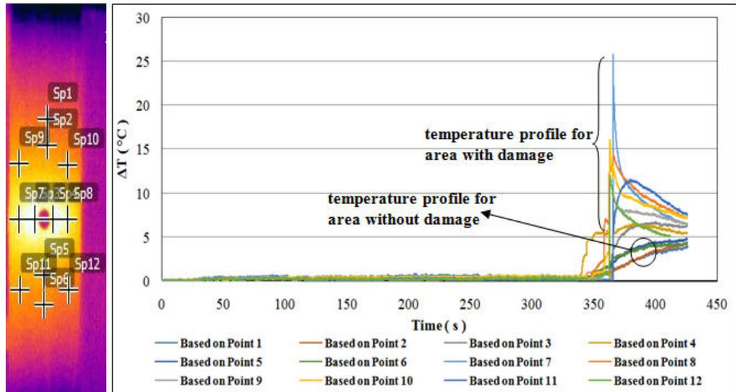
Figure 4.16 Temperature evolution of GFRP 0° with hole
