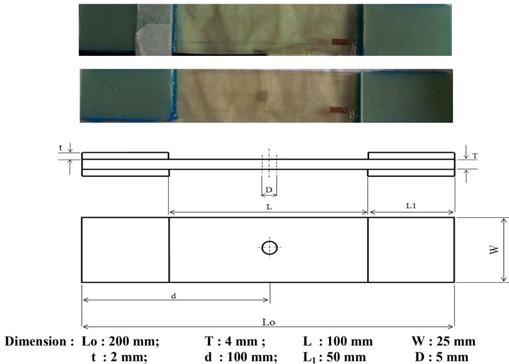
Figure 3.1 GFRP specimen
