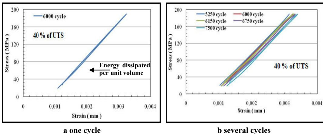
Figure 5.34 Energy dissipation under 40% of UTS fatigue loading of DCFC
