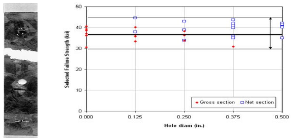
a. Failure in gross section      b. Variation of notch strength with hole diameter
