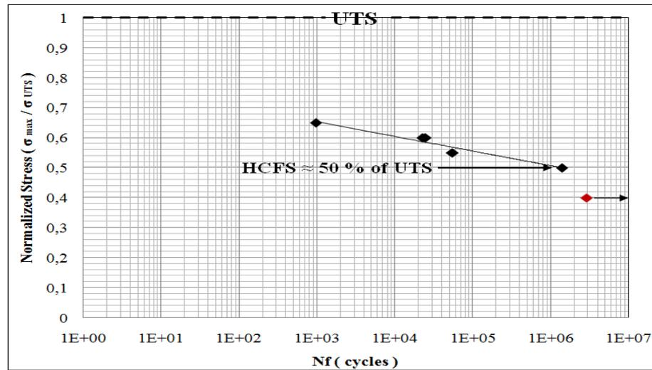
Figure 4.17 S-N curve for GFRP 90° with hole
