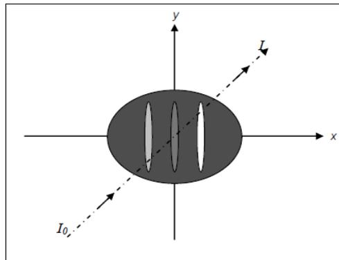
Figure 2.30 An X-ray beam passing through an object with different four linear attenuation coefficients [78]
