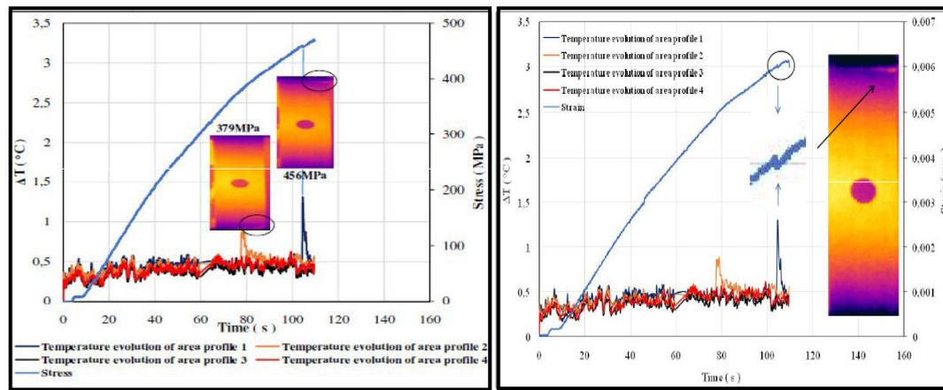
Figure 5.25 Temperature and stress-strain evolution during the test
