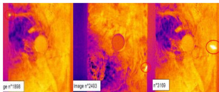
Figure 5.15 Micro defects at the edge of the specimen of DCFC
