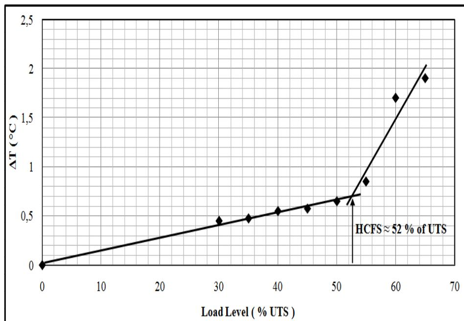
Figure 4.25 HCFS of GFRP  $90^{\circ}$  by thermography method
