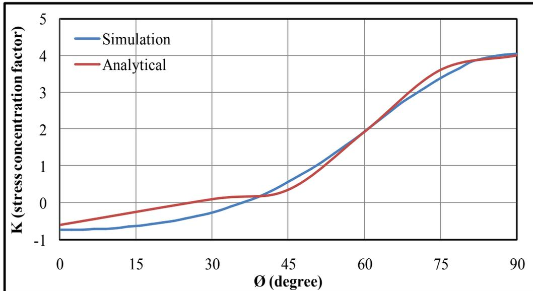
Figure D.7 Simulation vs analytical of  $K$  along the hole
