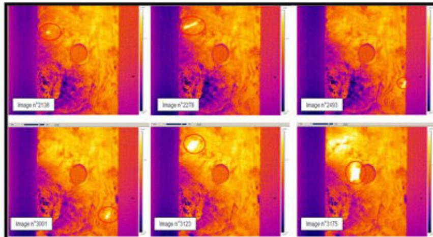
Figure 5.14 Delta-T spots of DCFC with an open hole specimen
