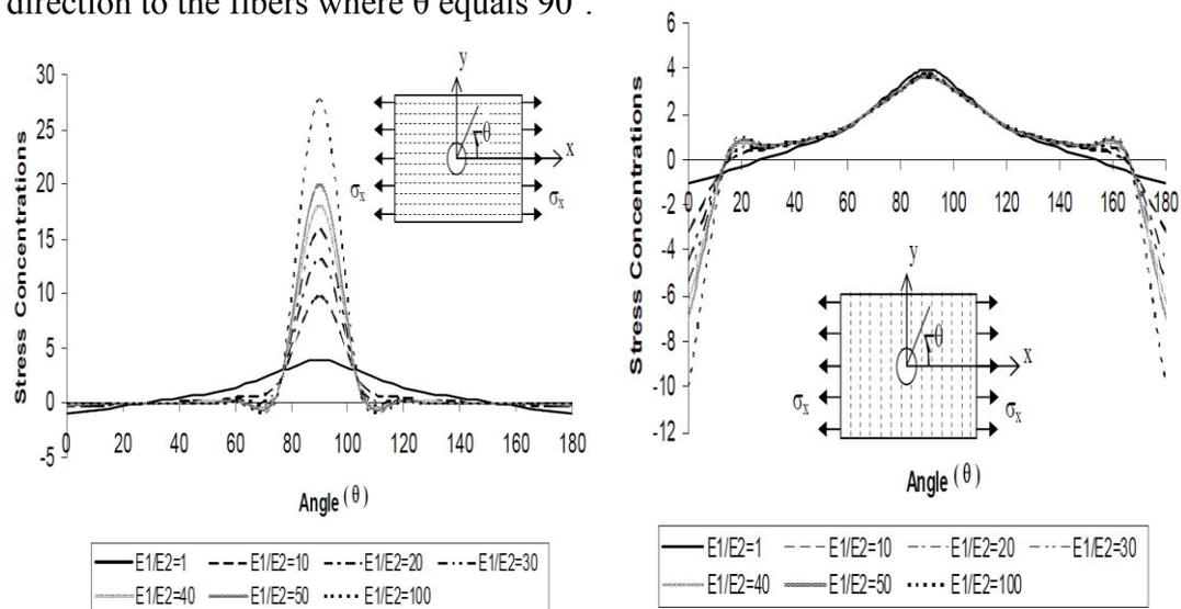
Figure 2.15 Stress concentration versus  $\theta$  for various elasticity modulus ratio [41]
