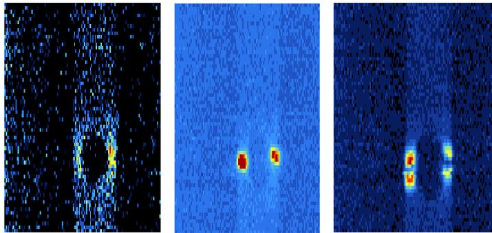
Figure 2.19 Thermography images of damage mechanism on composite [34]
