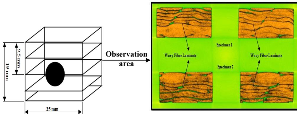
Figure 6.17 Wavy fiber laminate of GFRP 0°
