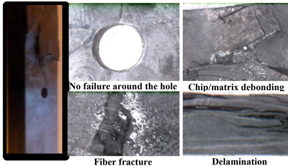
Figure 5.13 Damage type of DCFC under tensile loading
