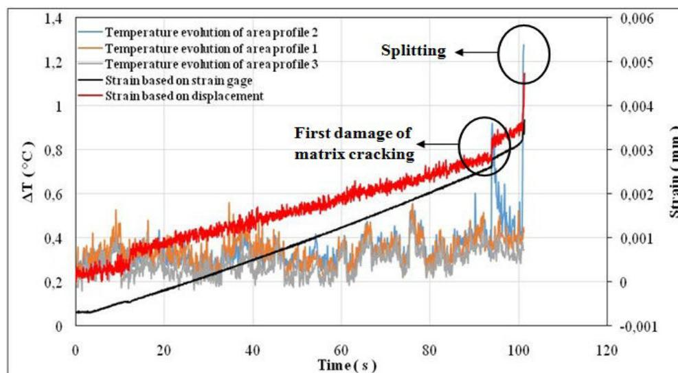
Figure 4.5 Strain and temperature evolution of GFRP  $90^{\circ}$  without hole
