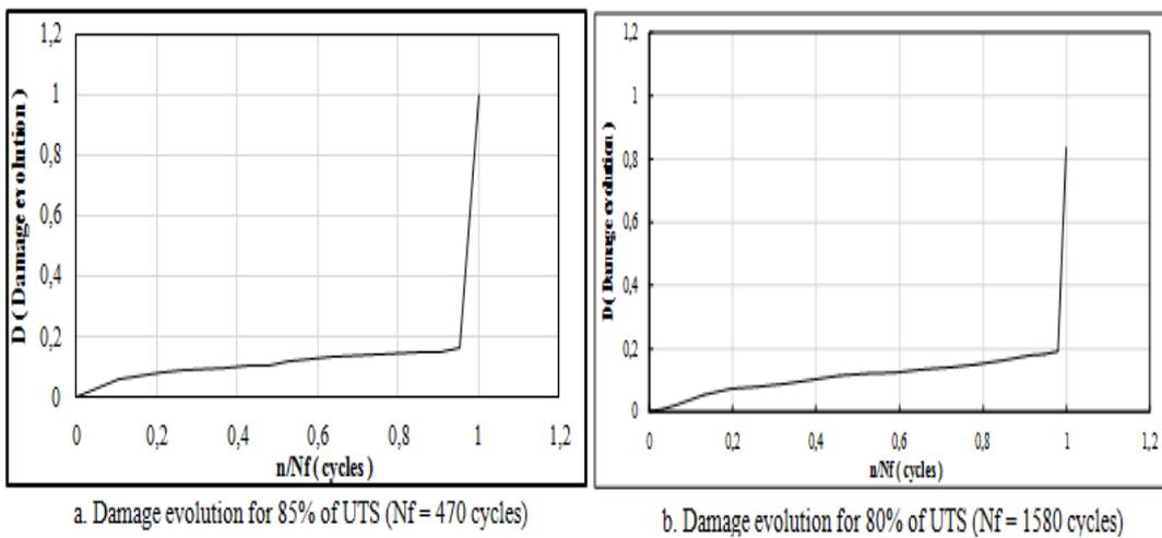
Figure 5.27 Damage evolution of DCFC
