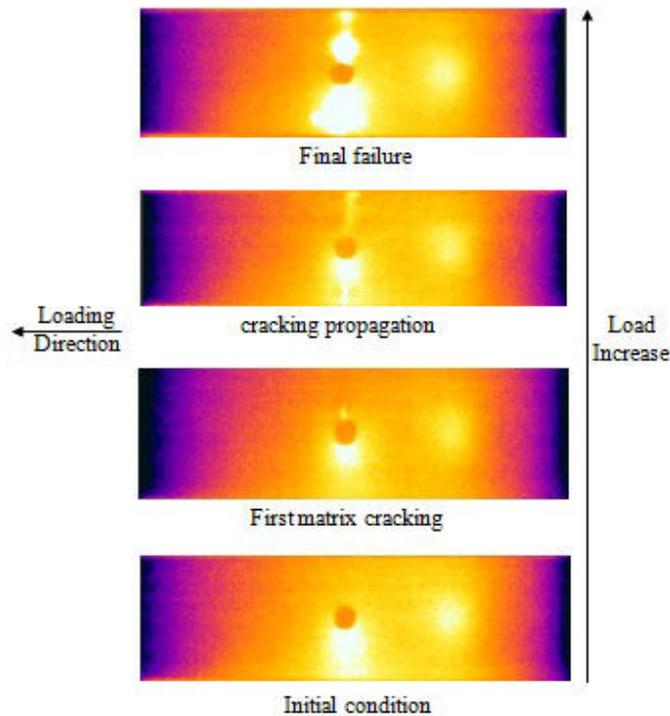
Figure 4.8 Thermography images of GFRP 90° with hole
