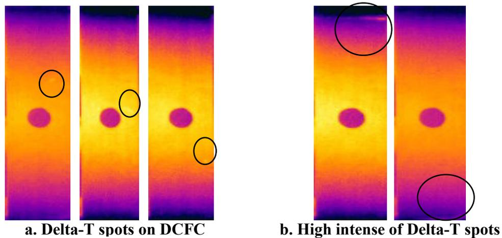
Figure 5.22 Delta-T spots on DCFC with an open hole during tensile loading
