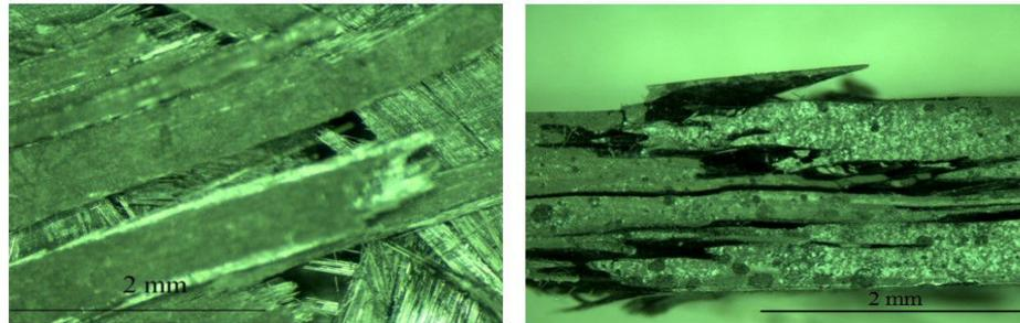
Figure 5.30 Rupture of DCFC specimen under fatigue loading
