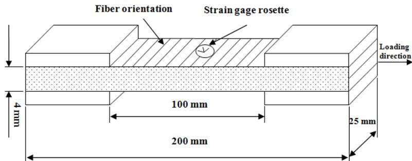
Figure A.1 Specimen of GFRP 90° and placement of strain gage rosette
