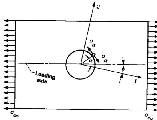
Figure 2.10 Tension at an angle to a principal elastic axis 1 of an isotropic plate with a hole [38]
