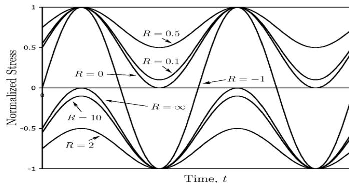
Figure 2.8 Different loading ratios to a maximum absolute value stress of 1.0
