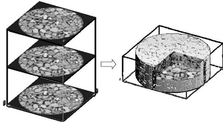
Figure 2.31 3D internal microstructure of a testing sample is reconstructed from series of x-ray tomography images [79].
