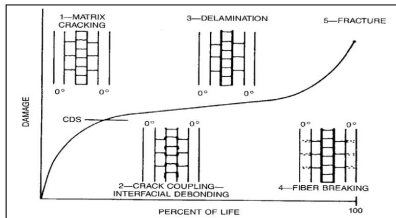
Figure 2.5 Development of damage in composite under fatigue [11]
