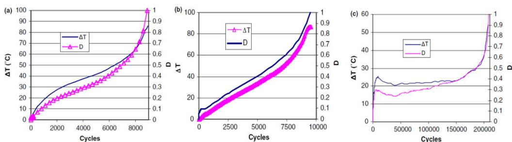
Figure 2.20 Comparison between the change of temperature and the damage evolution: (a) 70% level of loading, (b) 67.5% level of loading, (c) 60% level of loading [51]
