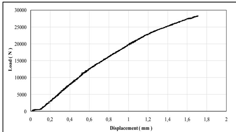
Figure 5.18 Tensile curve of DCFC with hole
