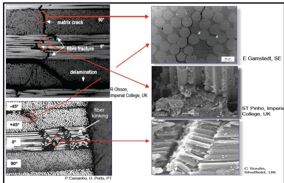
Figure 2.6 Damage type of fiber reinforced plastic [27]
