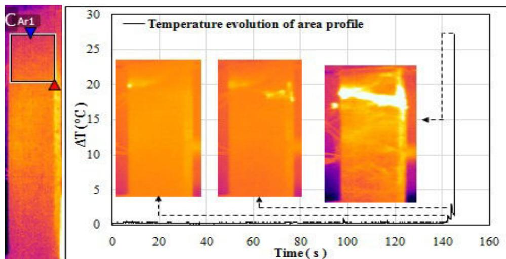
Figure 5.10 Temperature evolution at final failure period
