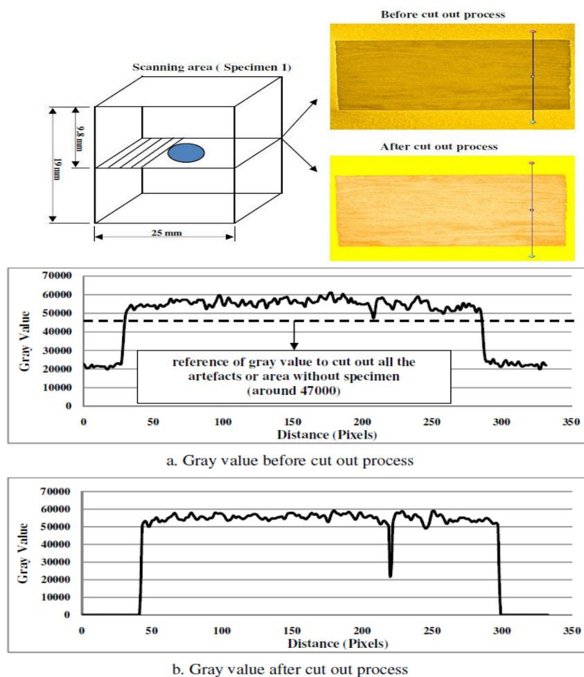
Figure 6.8 Cut out of gray value process of DCFC
