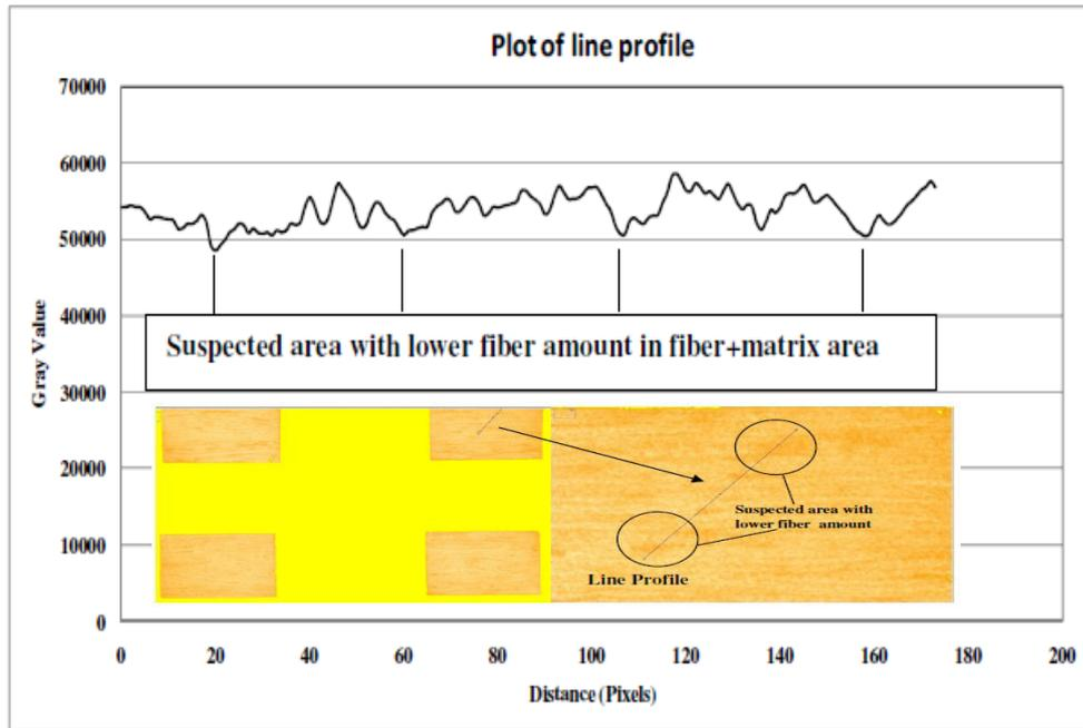
Figure 6.11 Gray value parameter of line profile for DCFC
