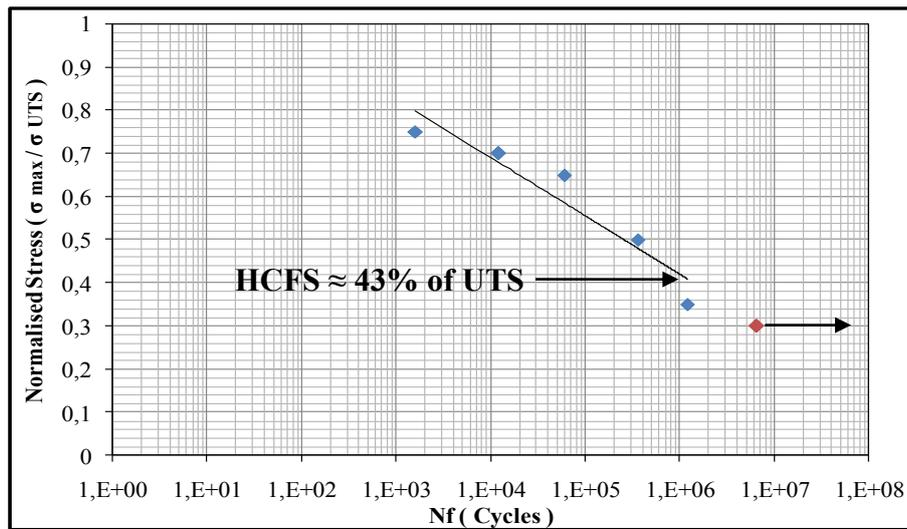
Figure 5.26 S-N curve of DCFC
