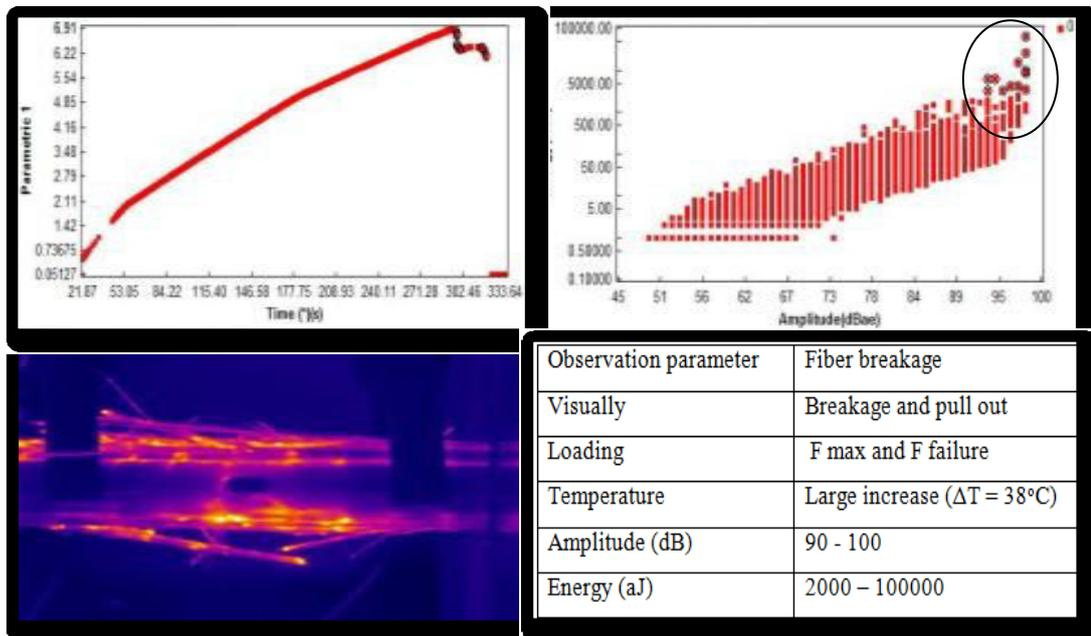
Figure 6.4 Observation results of fiber breakage and fiber pull out of GFRP  $0^{\circ}$  [95]
