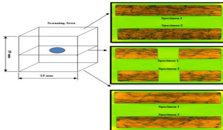
Figure 6.14 Example of slice image of GFRP 0° around the hole
