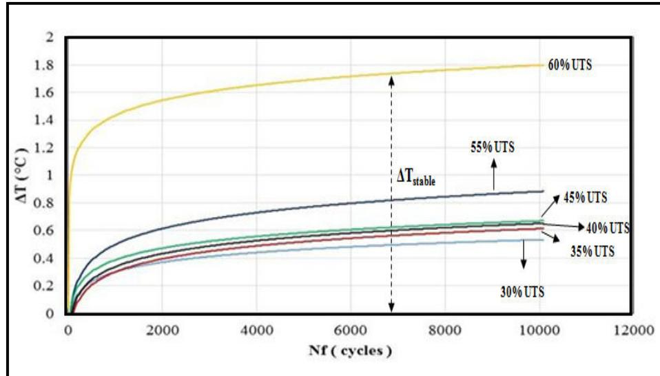
Figure 4.24 Temperature profile of GFRP  $90^0$  for each load level
