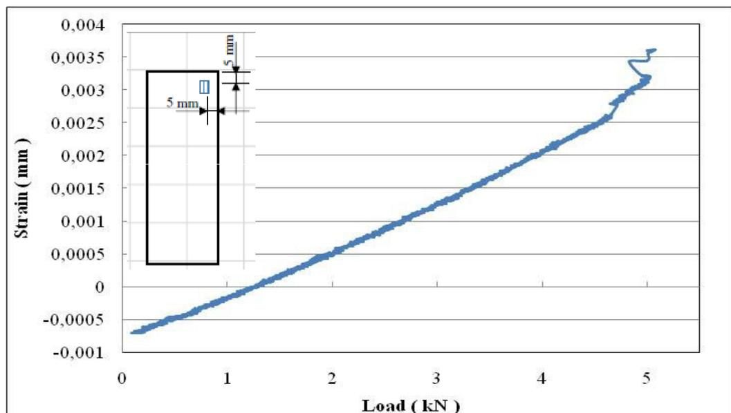
Strain of mechanical testing based on strain gage
