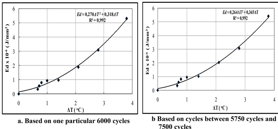
Figure 5.36 Energy dissipation versus  $\Delta T_{stable}$  of DCFC for different load level
