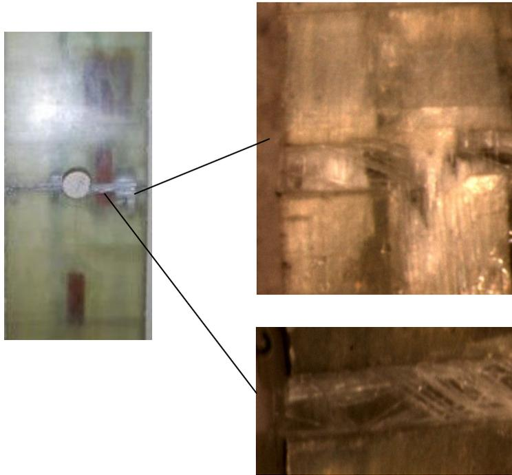
Figure 4.21 Final failure of GFRP 90° with hole under fatigue loading
