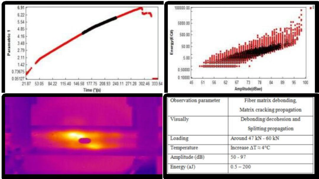
Figure 6.3 Fiber matrix debonding recorded by thermography and AE of GFRP 0° [95]
