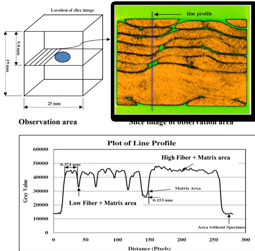
Figure 6.16 Gray value parameter of line profile for GFRP 0°
