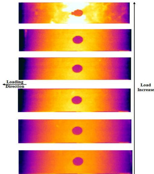
Figure 5.21 Thermography images of DCFC specimen with open hole
