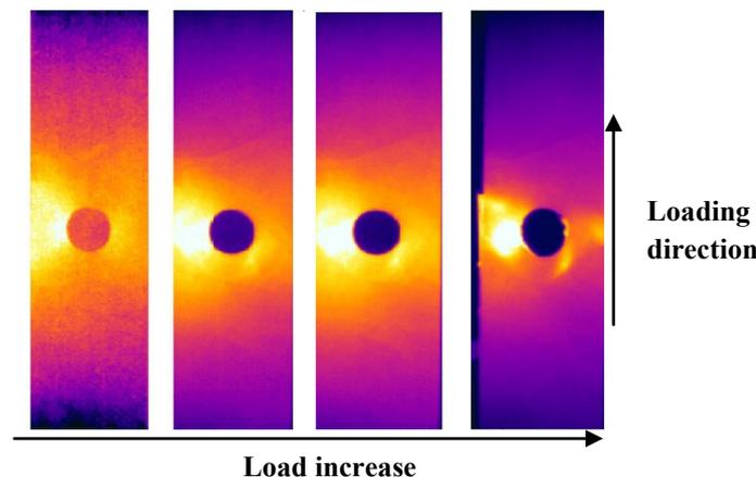
Figure 5.29 Thermography images of DCFC under fatigue test with 80% of UTS
