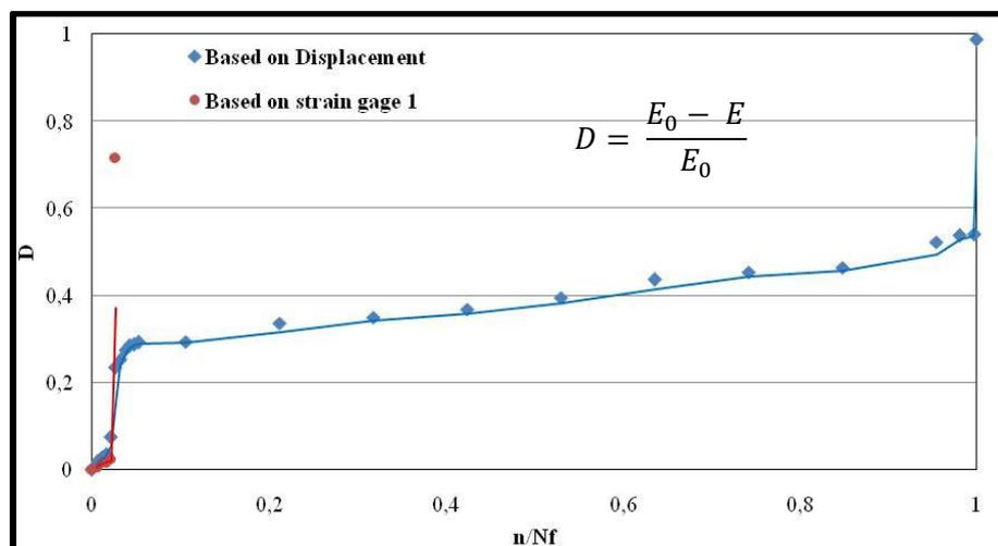
Figure 4.20 Damage evolution of GFRP 90° with 65% of UTS
