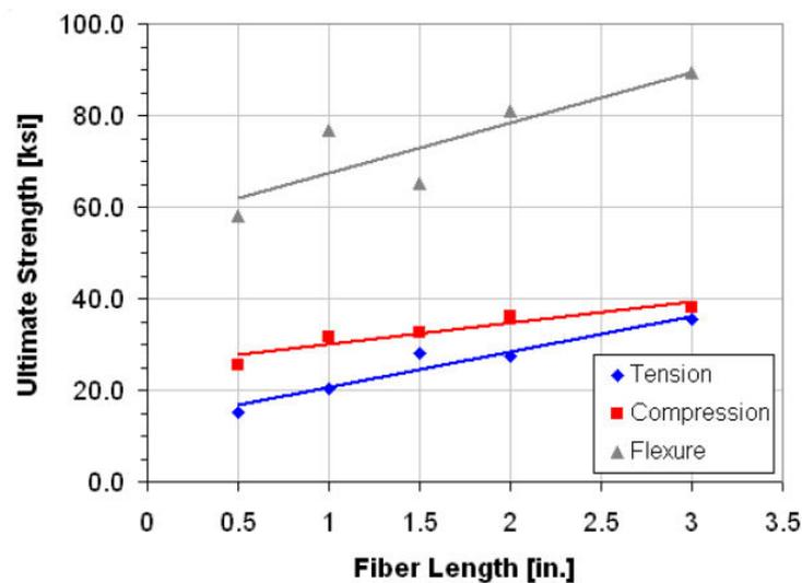
Figure 2.40 UTS of DFC for different static condition [86]
