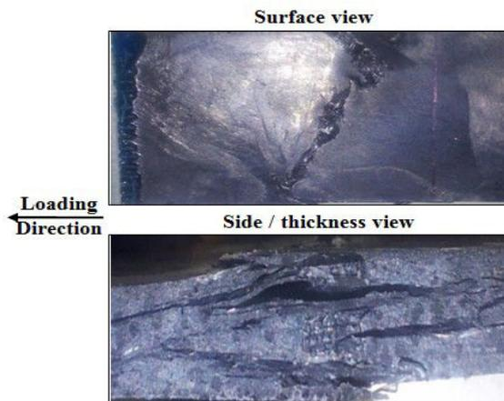
Figure 5.3 Catastrophic damage form of DCFC under tensile loading
