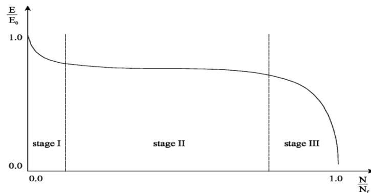
Figure 2.4 Stiffness degradation of fiber reinforced composite materials [13]
