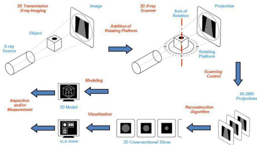
Figure 2.29 Overview of CT scan and measurement process [77]
