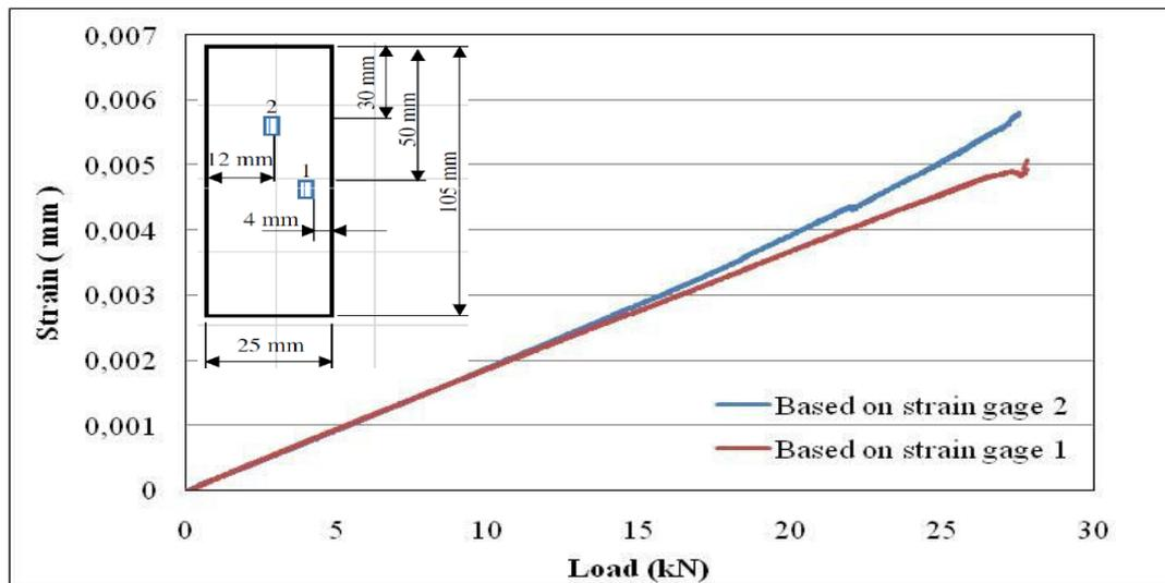
Strain of mechanical testing based on strain gage
