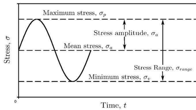
Figure 2.7 Illustration of sinusoidal loading
