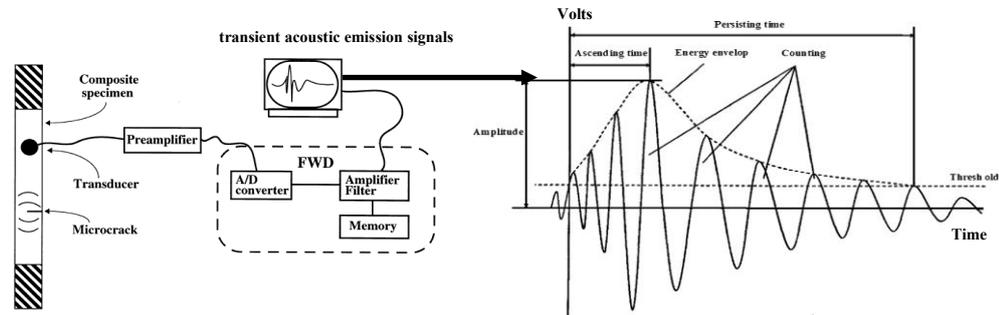
Figure 2.24 Acoustic Emission Illustration [69]
