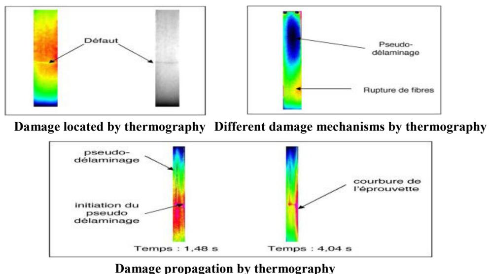
Figure 2.22 Damage observation by thermography on carbon fiber composite [52]
