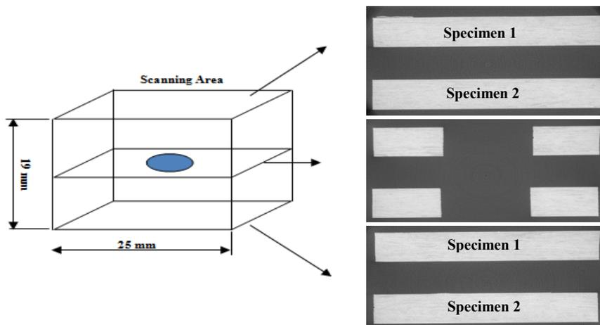
Figure 6.6 Example of slice image of DCFC resulting by CT-Scan around the hole
