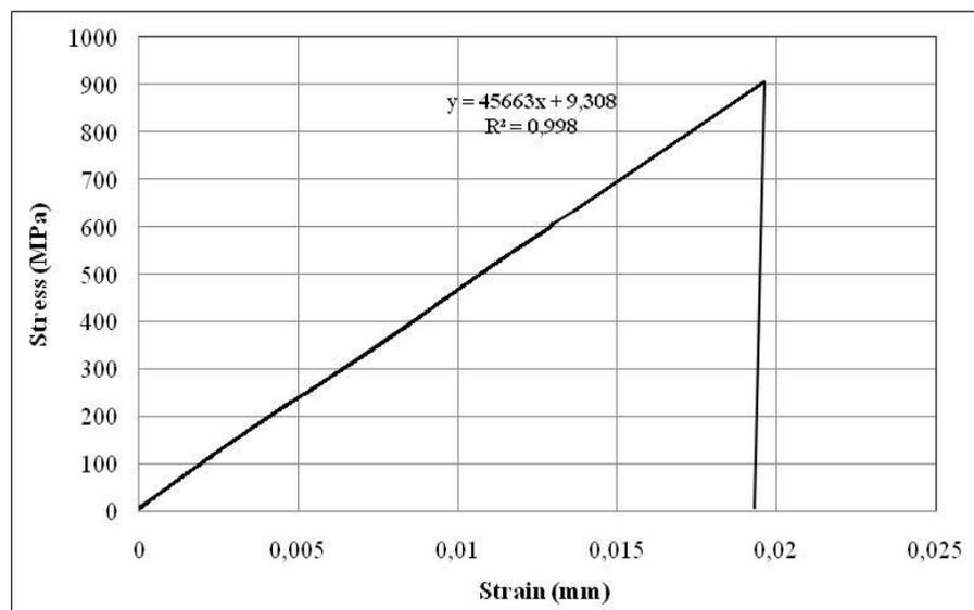
Figure 4.11 Tensile curves of GFRP 0° with hole
