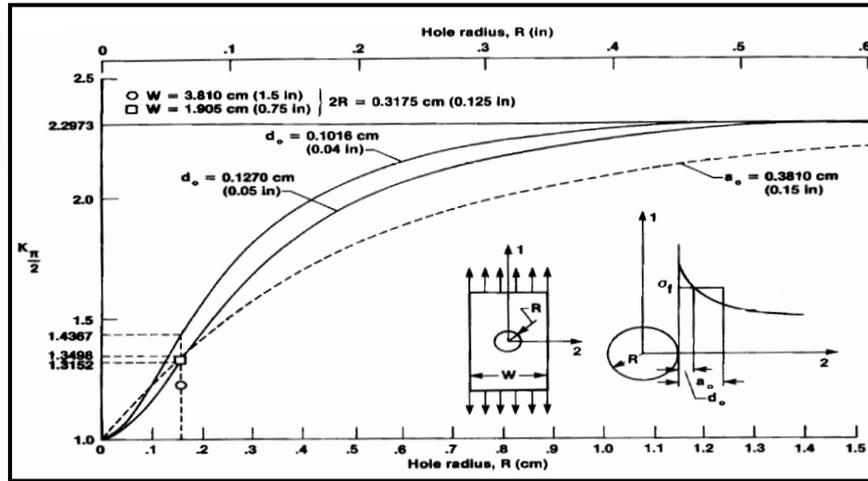
Figure 2.13 Stress concentration factor  $K_{\pi/2}$  as a function of hole size
