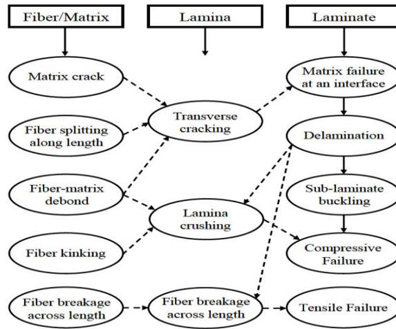
Figure 2.9 Failure mode at different scales
