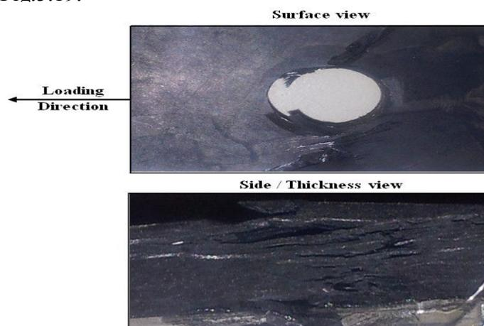
Figure 5.19 Damage form of DCFC with an open hole
