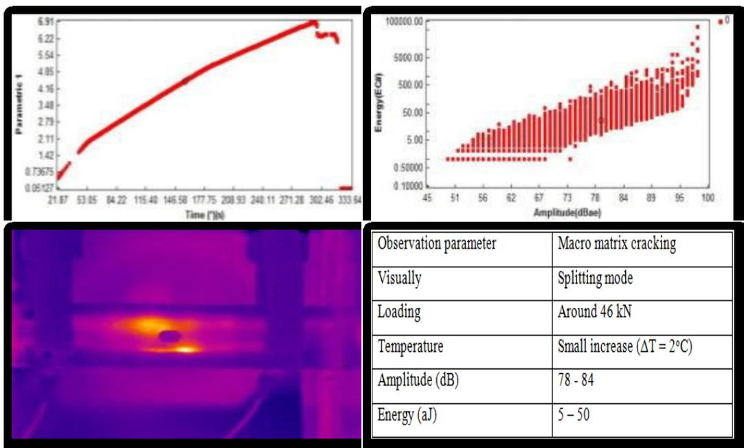
Figure 6.2 Thermography and AE results of first damage under tensile test of GFRP 0° [95]
