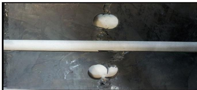
Figure 5.17 Rupture of DCFC with D/W ratio of 0.4
