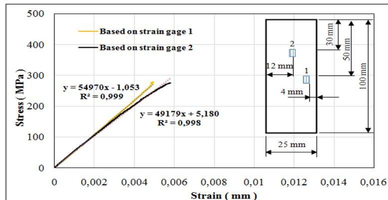
Figure 5.4 Stress-strain curve of DCFC specimen
