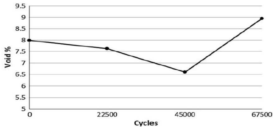
Figure 2.36 Micro-voids percentage in the entire samples as a function of the fatigue life (number of cycles) [82].
