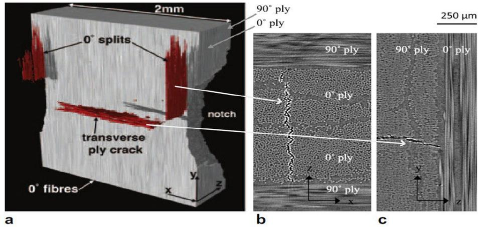
Figure 2.32 Tomography 3D visualization of damage on composite material [80]
