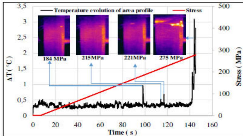
Figure 5.9 Stress and temperature evolution of DCFC
