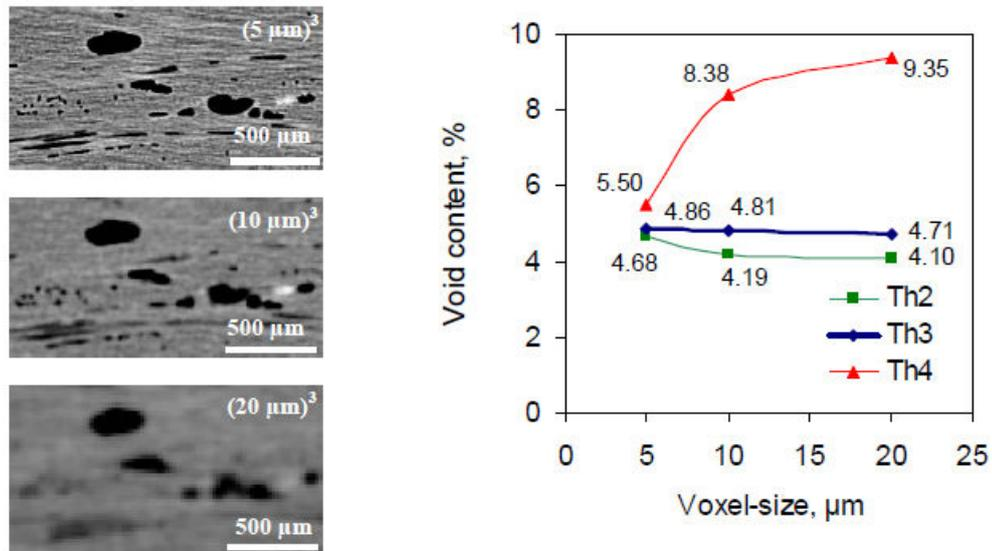
Figure 2.34 CT images of a sample measured with different voxel sizes [81]
