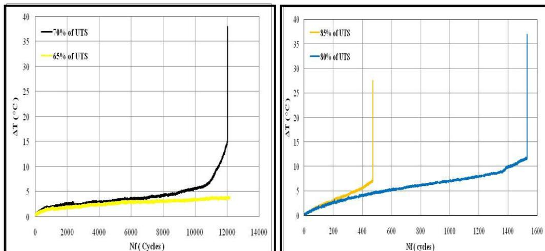
Figure 5.28 Temperature profile during fatigue test for each different load level
