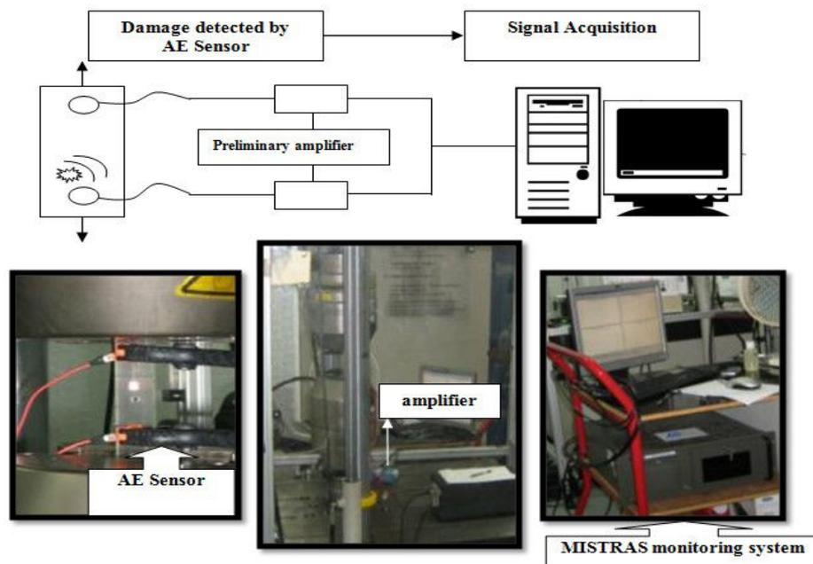
Figure 3.4 Acoustic Emission set up
