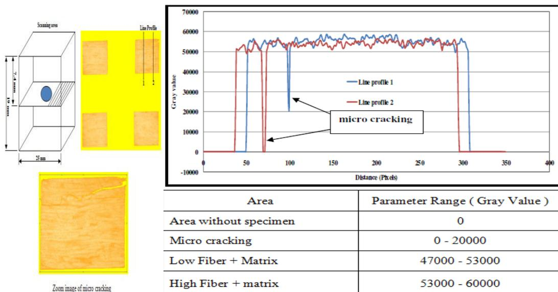
Figure 6.12 Gray value parameter of line profile for micro cracking on DCFC
