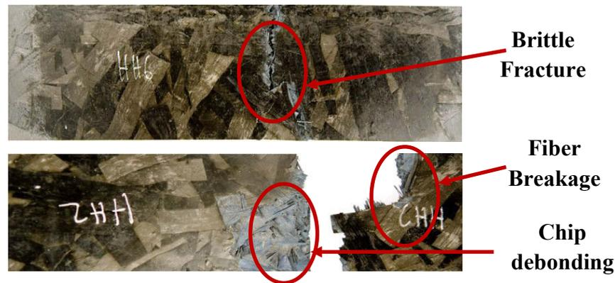
Figure 2.41 Failure of DCFC [87]
