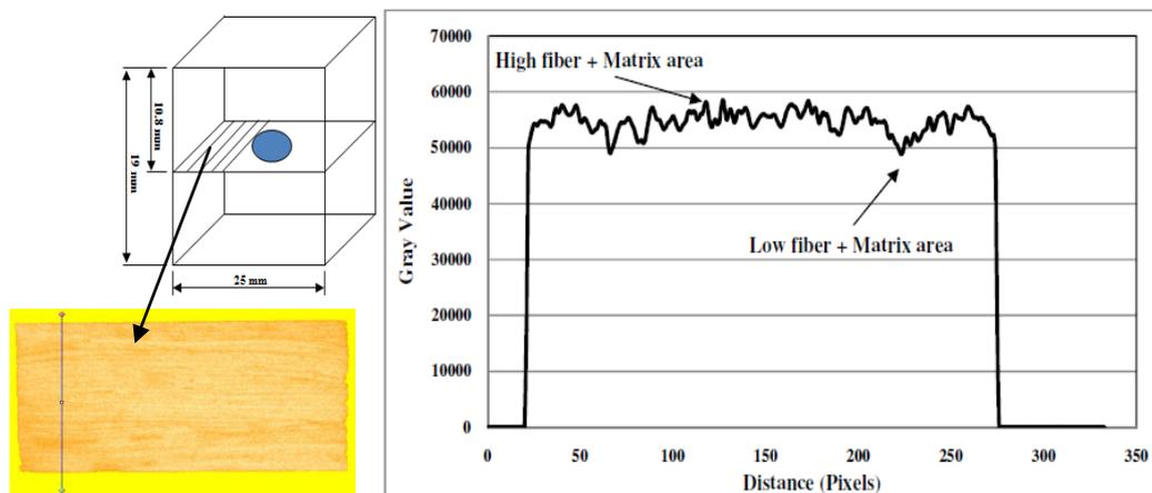
Figure 6.10 Gray level parameter of line profile for DCFC
