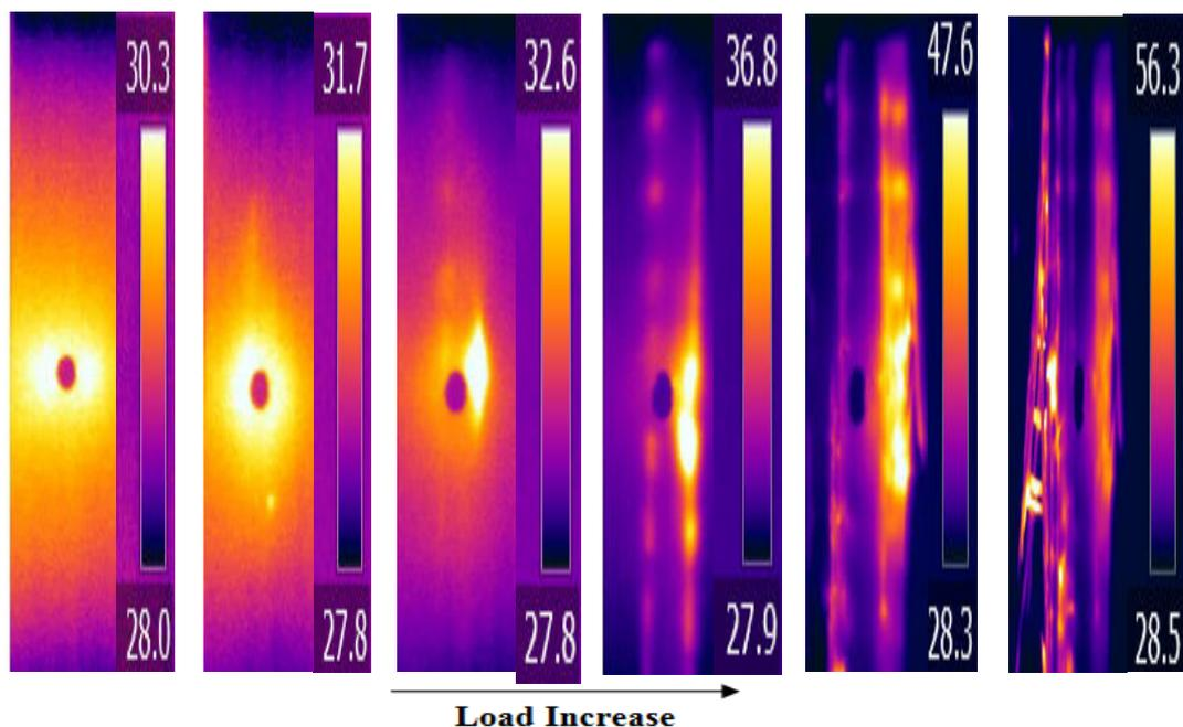
Figure 4.15 Thermography images of GFRP 0° with hole
