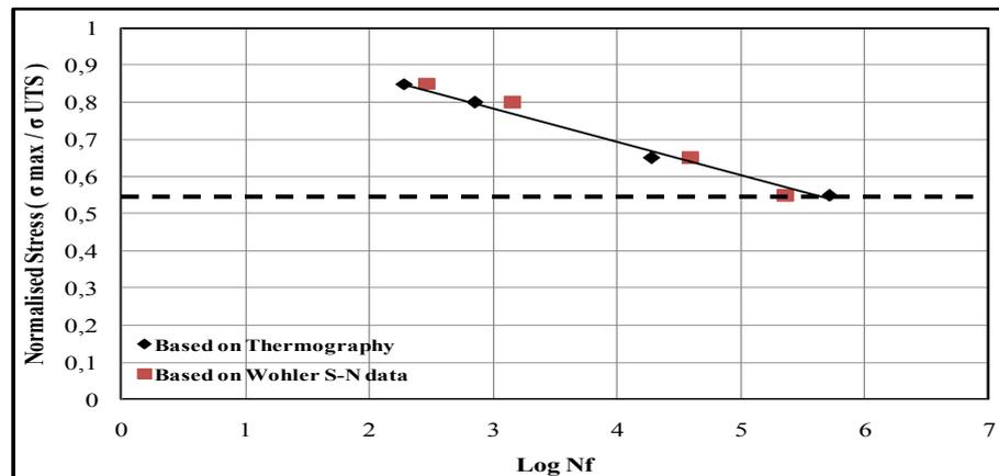
Figure 5.37 S-N curve of DCFC based on thermography approach using  $\Phi$  parameter
