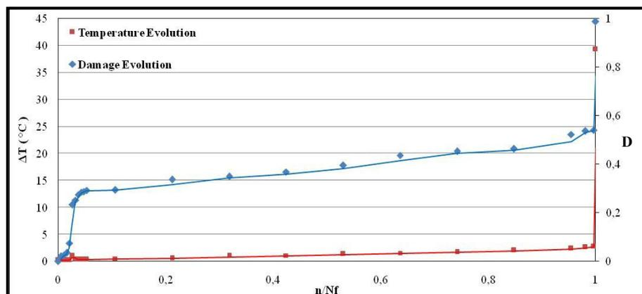
c. Temperature and damage evolution until rupture
