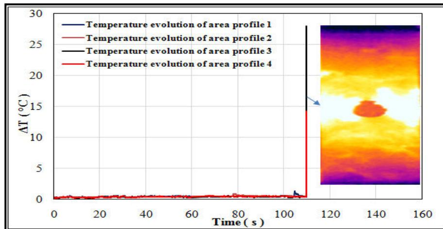
Figure 5.24 Temperature evolution on specimen surface until final failure
