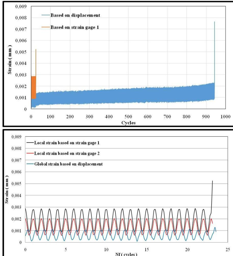
Figure 4.18 Strain propagation of GFRP 90° during the test
