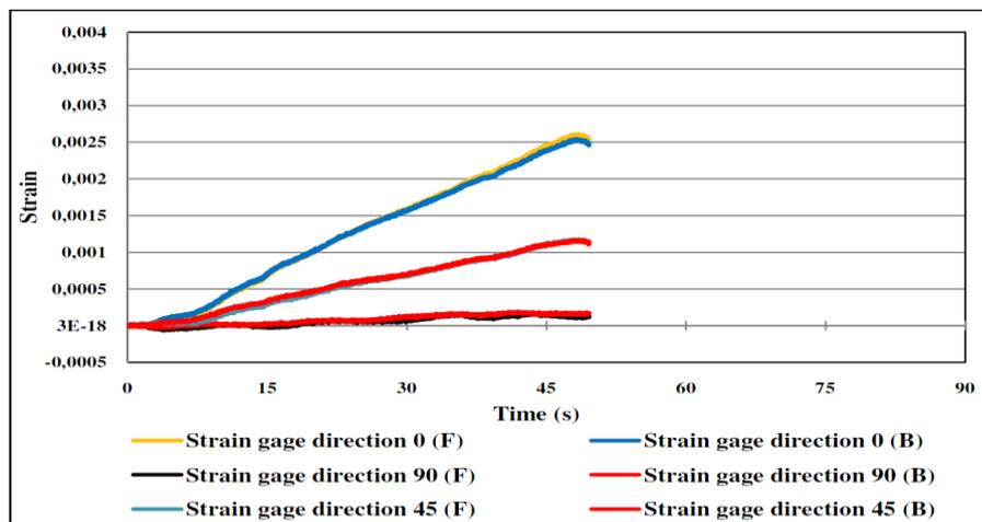
Figure A.2 Strain propagation of GFRP 90° during tensile test
