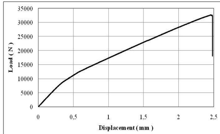
Figure 5.11 Tensile curve of DCFC with hole
