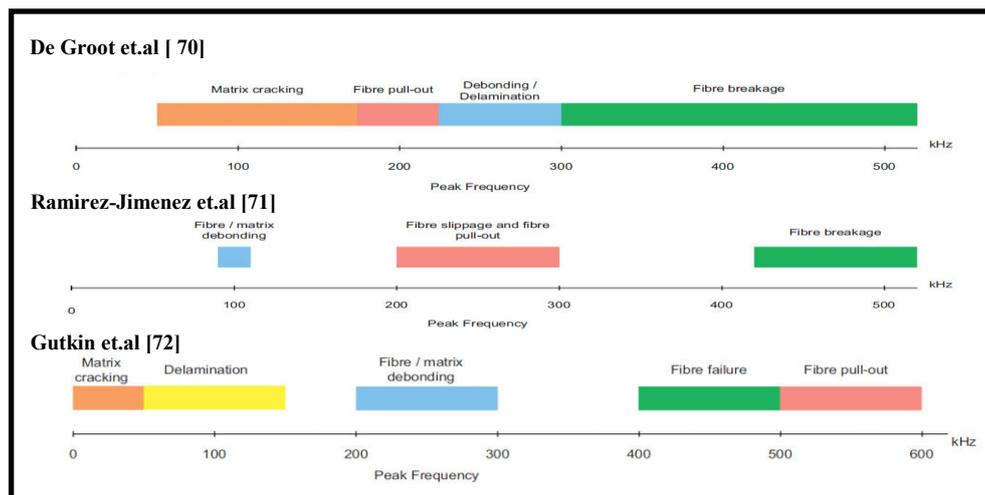
Figure 2.25 Frequency domain of acoustic emission of composite damage
