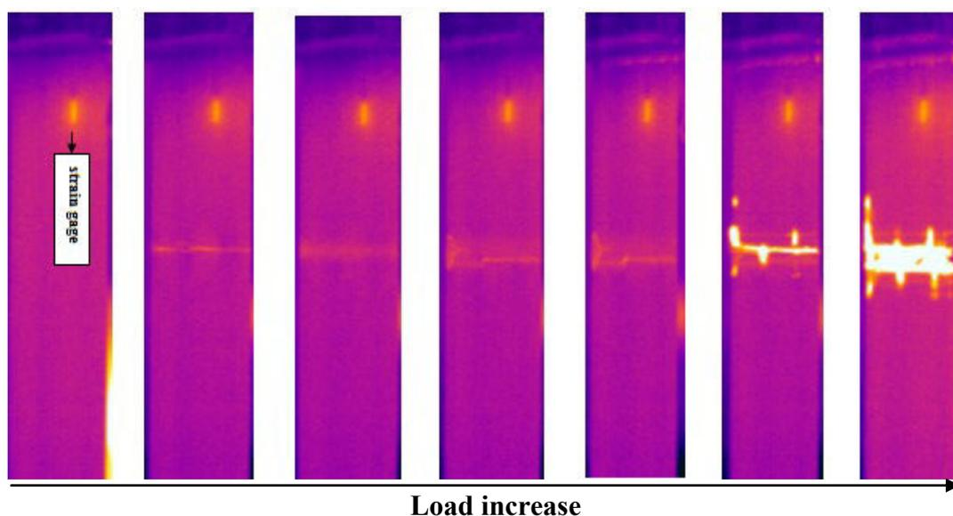
Figure 4.3 Thermography images of GFRP 90° without hole
