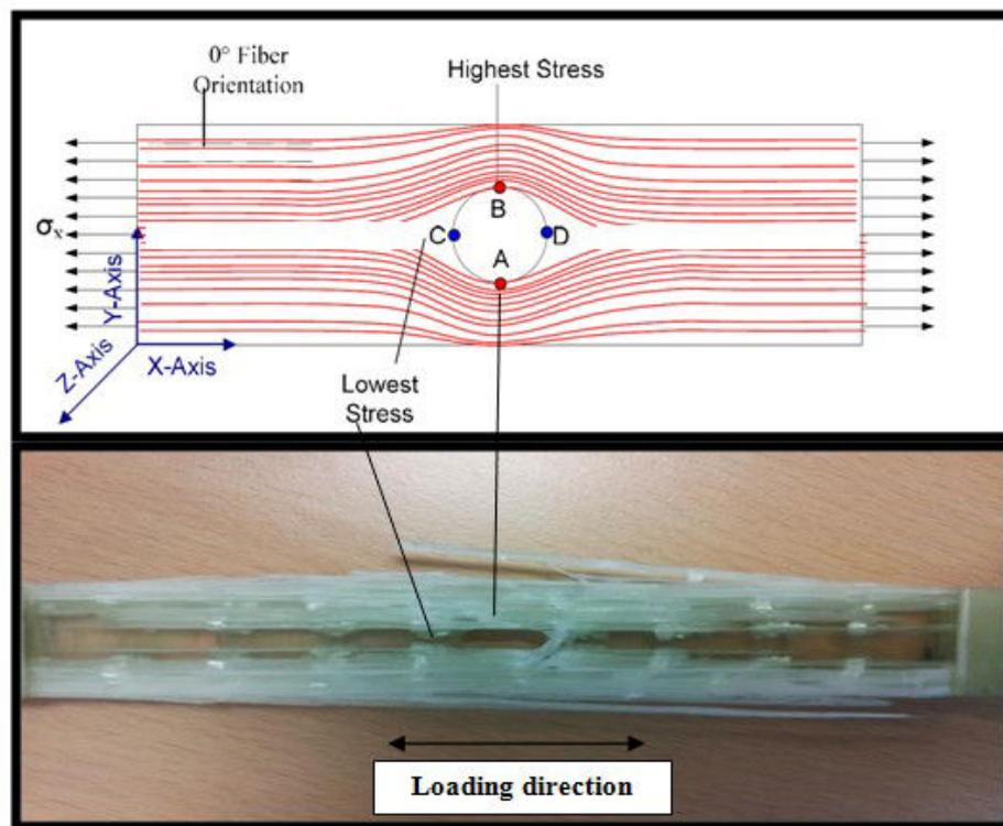
Figure 4.13 Illustration of stress distribution and final failure of GFRP  $0^\circ$
