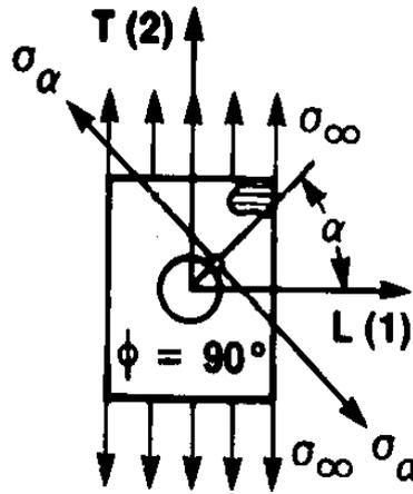
Figure D.3. Illustration of the loading direction GFRP  $90^\circ$
