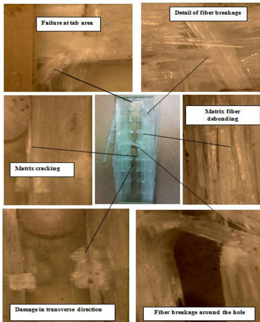
Figure 4.14 Damage types of GFRP 0° with hole
