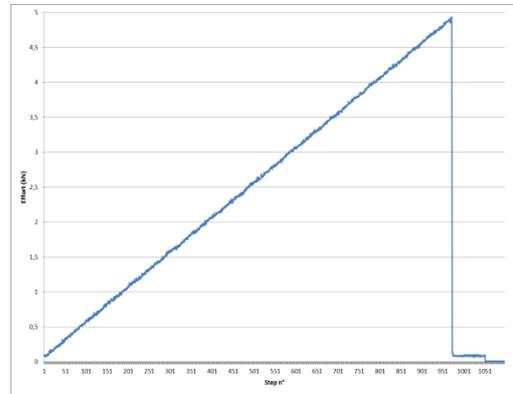
Load of mechanical testing
