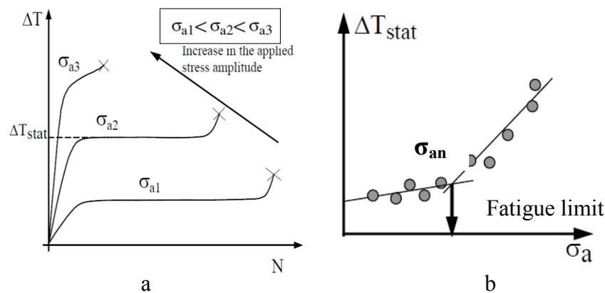
Figure 2.23 (a) Stabilisation temperature during fatigue test
