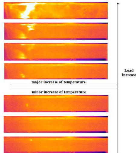
Figure 5.6 Thermography images of DCFC without hole
