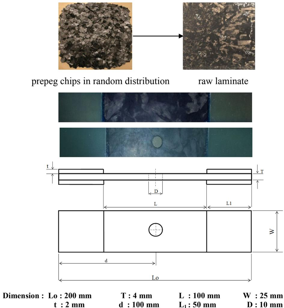
Figure 3.2 DCFC specimen
