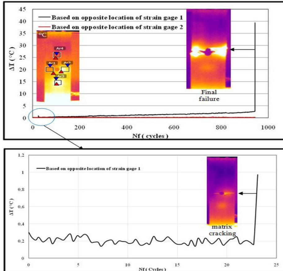
Figure 4.22 Evolution of surface temperature of GFRP 90°
