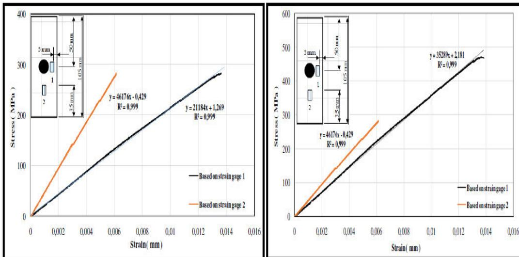
a. Stress-strain curve of DCFC
