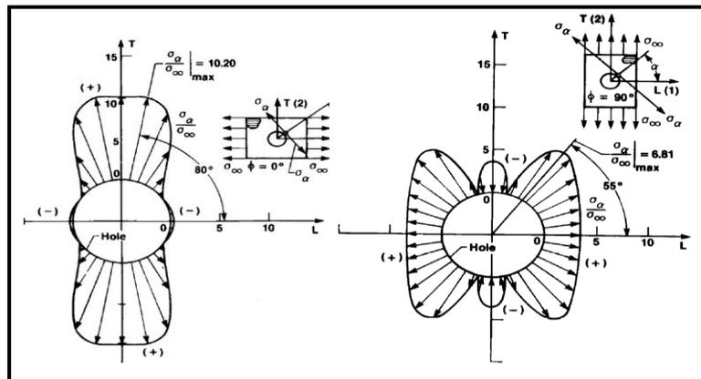
Figure 2.11 Tangential stress distribution around a hole [38]
