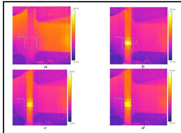
Figure 2.18 Temperature distribution during extension [43].
