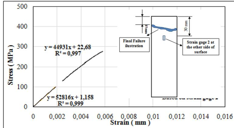
Figure 5.5 Change of modulus measurement of DCFC
