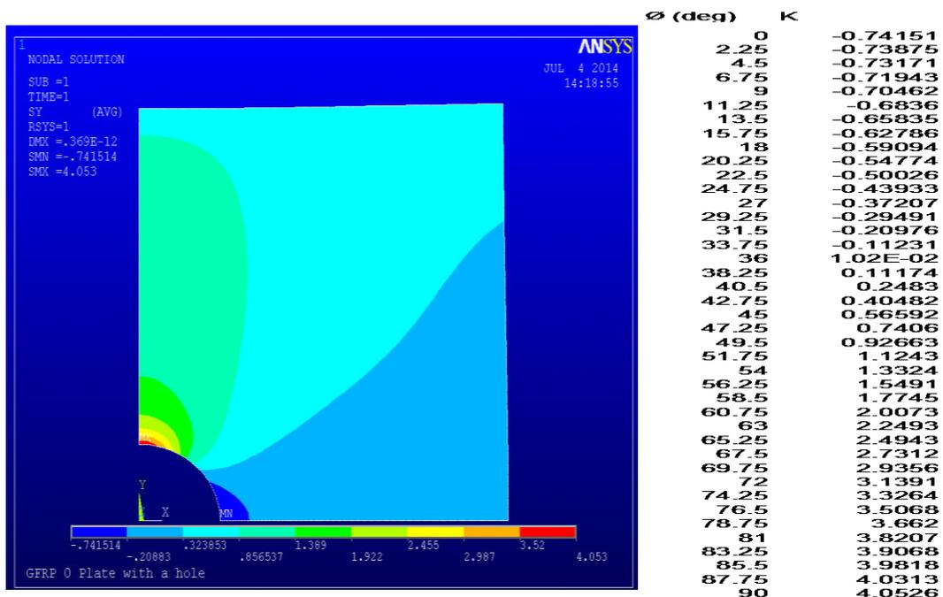
Figure D.6 Ansys model of stress distribution
