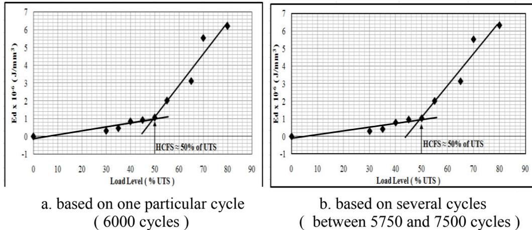
Figure 5.35 HCFS of DCFC by energy dissipation
