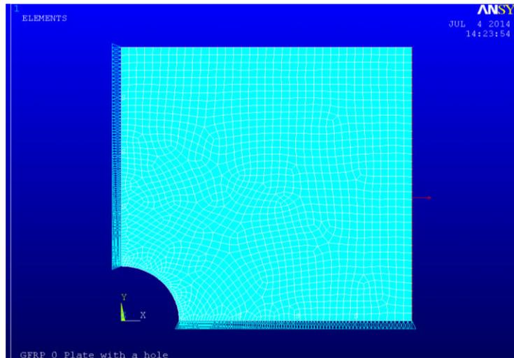
Figure D.5 Boundary conditions of the region to be modeled
