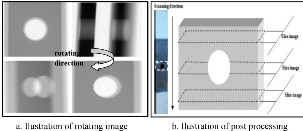
Figure 6.5 Illustration of CT scanning process
