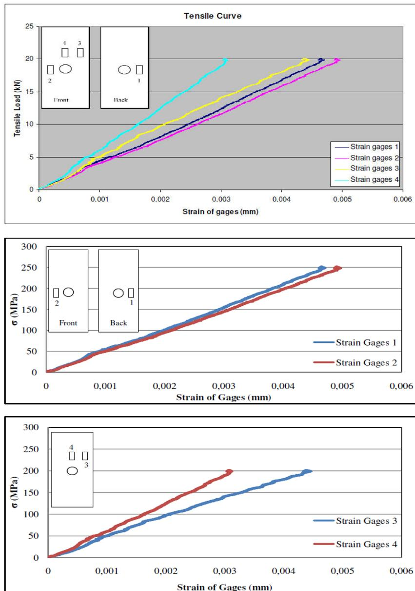
Figure 4.12 Tensile test of GFRP 0° with strain gage
