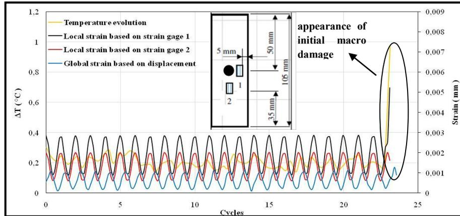
a. Temperature and strain gage detection on first macro matrix cracking
