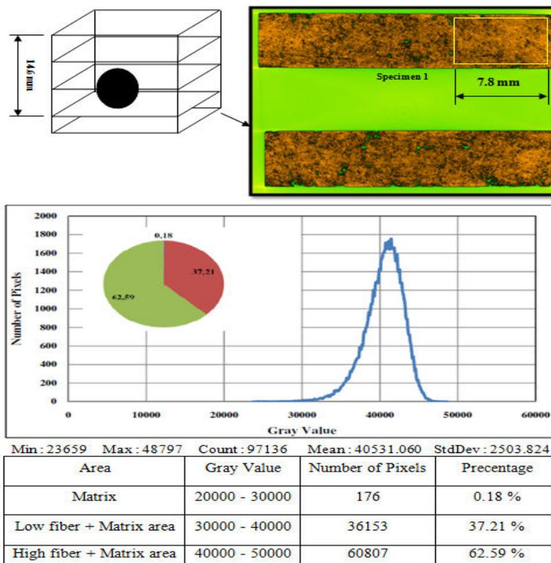
Figure 6.19 Histogram of slice image for GFRP 0°
