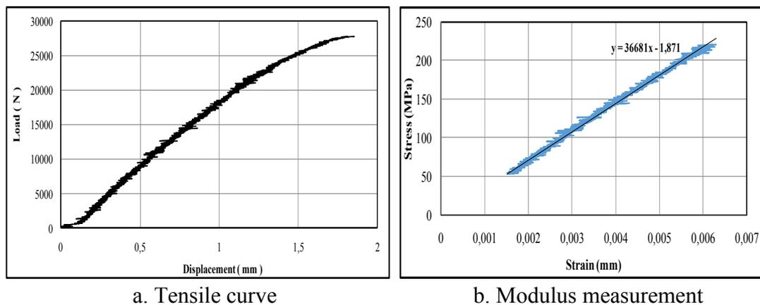
Figure 5.2 Tensile curve of DCFC
