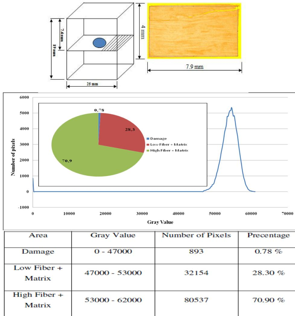
Figure 6.13 Histogram of slice image of DCFC
