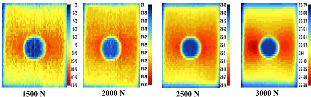
Figure 2.21 Temperature changes as increase of stress around the hole on CFC under tension compression fatigue loading [50]
