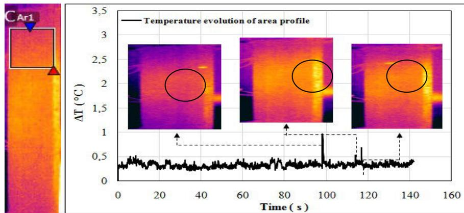
Figure 5.7 Delta-T spots of DCFC specimen during tensile loading
