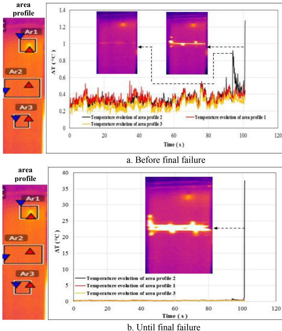
Figure 4.4 Temperature evolution of GFRP 90° without hole
