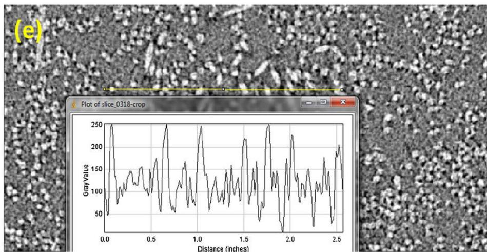
Figure 2.35 Grey value along the yellow line parameter with fibers are shown white and voids black [82]
