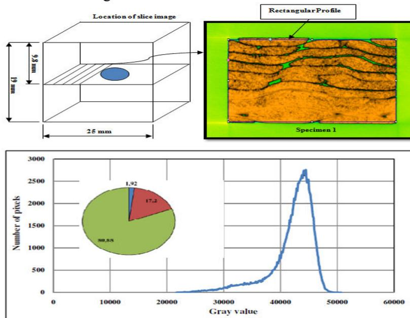
Figure 6.18 Histogram of slice image from GFRP 0°
