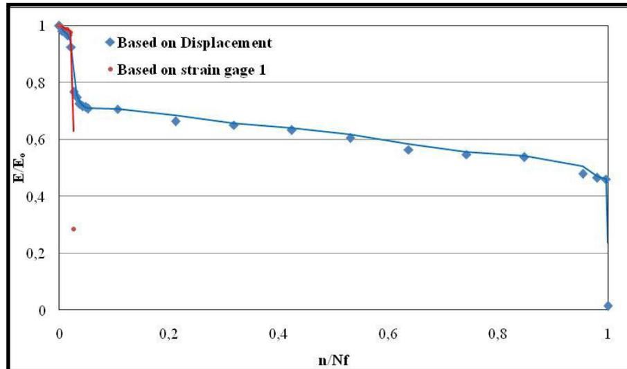
Figure 4.19 Normalized Stiffness degradation at 65% UTS tests of GFRP 90°
