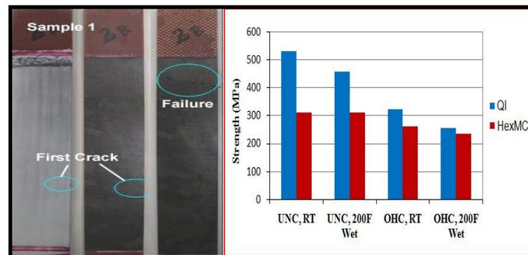
Figure 2.39 Failure and insensitive of DCFC [85]
