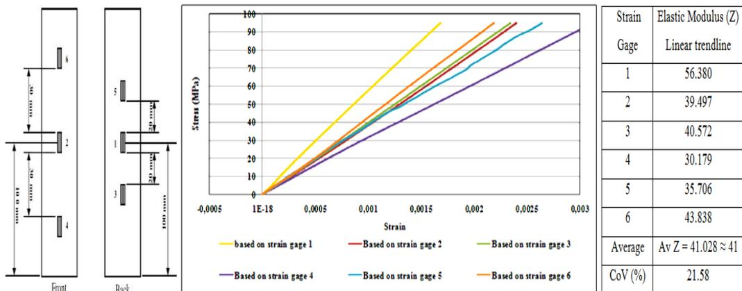
Figure 5.1 Stress-strain curve of DCFC without hole
