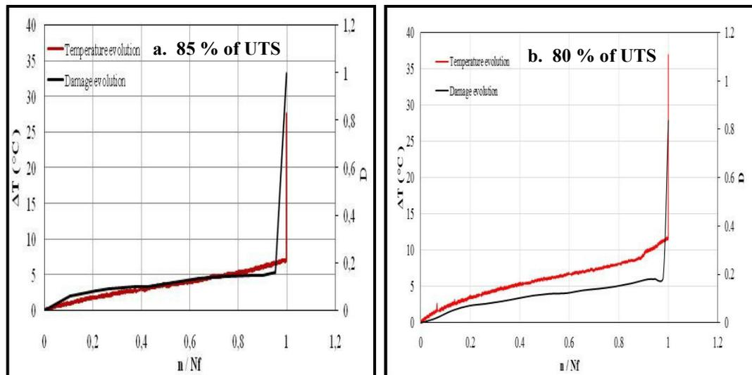
Figure 5.31 Comparison between the temperature and the damage evolution
