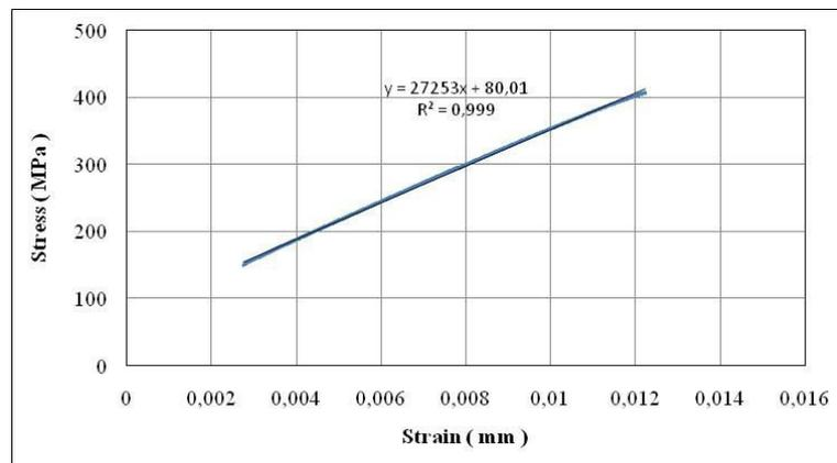
Figure 5.12 Stress - strain curve of DCFC specimen
