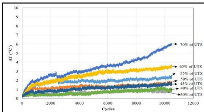
Figure 5.32 Temperature profile of DCFC for each load level
