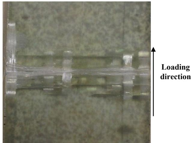
Figure 4.2 Macroscopic of catastrophic damage form of GFRP 90° without hole
