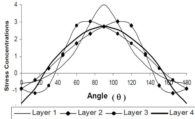
Figure 2.14 Stress concentration factor versus  $\theta$  for glass-epoxy composite
