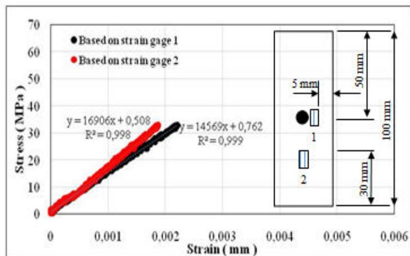
Figure 4.6 Stress-strain curve of GFRP 90° with hole
