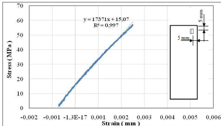
Figure 4.1 Stress-strain curve of GFRP 90° without hole
