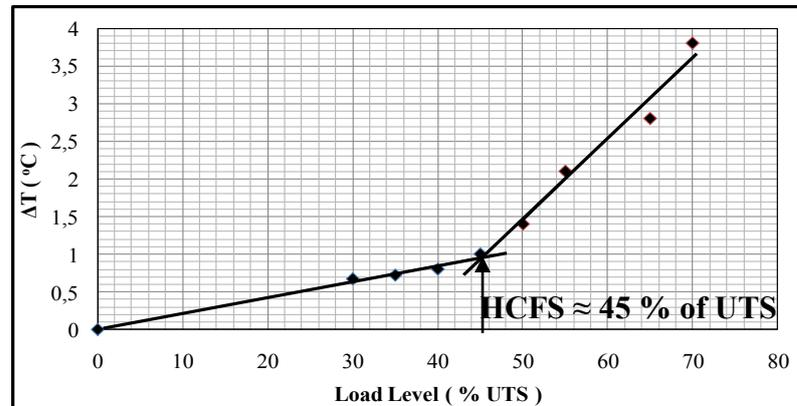
Figure 5.33 HCFS of DCFC by thermography method
