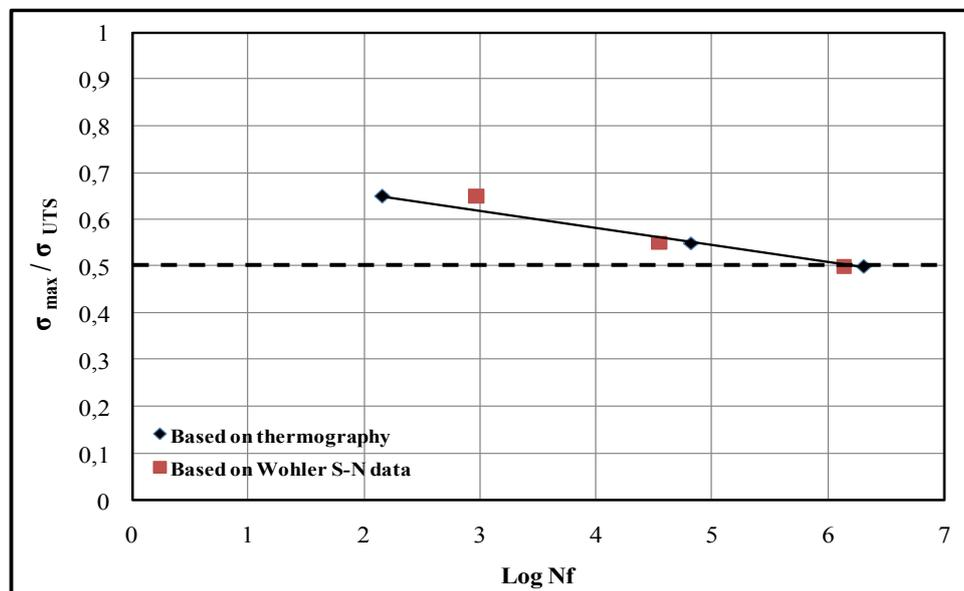
Figure 4.29 S-N curve based on thermography approach using  $\Phi$  parameter
