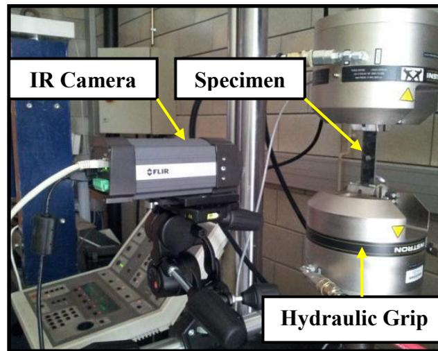
Figure 3.3 INSTRON Machine and IR camera
