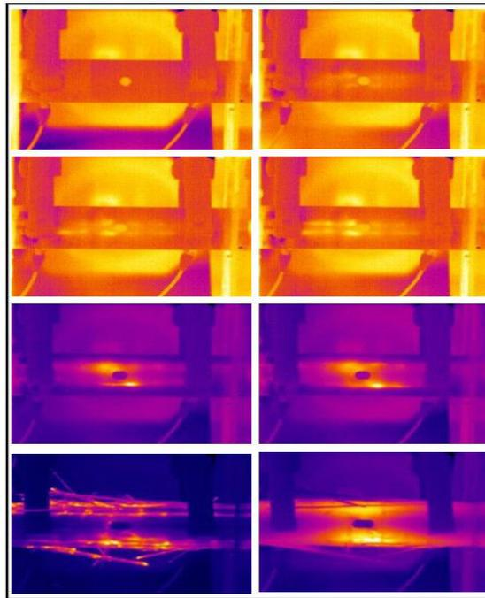
Figure 6.1 Thermography images of GFRP 0°
