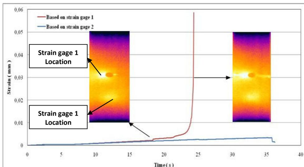
Figure 4.10 Macro damage detection by strain gage and thermography
