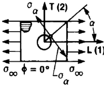
Figure D.4 Illustration of the loading direction GFRP  $0^\circ$
