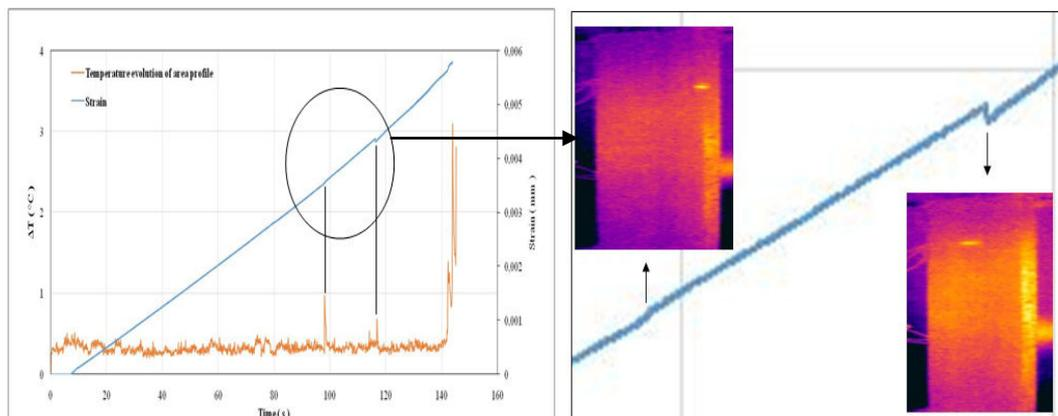
Figure 5.8 Strain and temperature evolution of micro damage of DCFC
